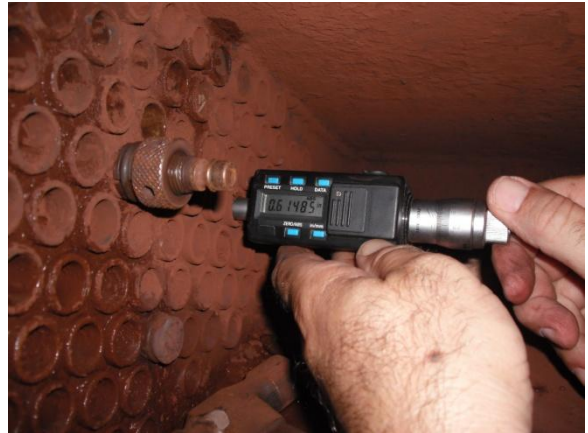
Figure 4 - Measuring inlet tube ID profiles for signs of inlet end erosion
