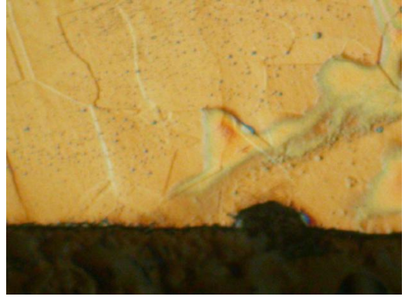
Figure 14 - Tube Defect viewed under microscope
