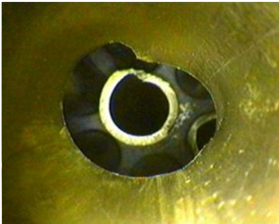
Figure 5 - Severed tube discovered by tube side video probe
