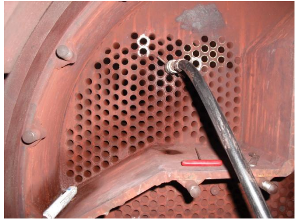
Figure 10 - Hydrotesting an individual tube to high pressure
